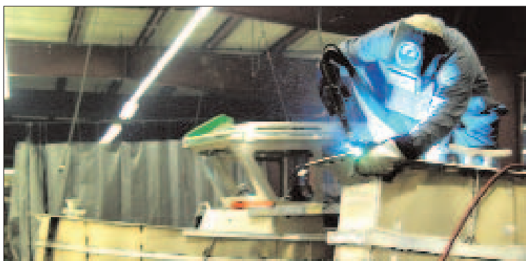
Dago Casas, a SAFE Boat International metal fabricator, welds a seam on the bow of one of the new Defender Class boats.
